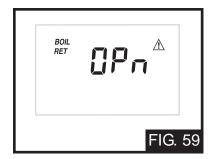
The control is no longer able to read the boiler return sensor due to an open circuit (FIG. 59). The control will continue to operate normally. Locate and repair the problem as described in INS7141. To clear the error message from the control after the sensor has been repaired, press either the Menu or Item button.
